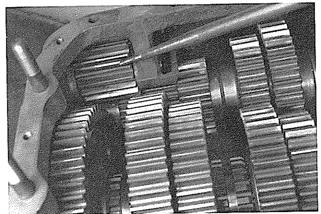
5. Roll the upper reverse idler gear toward the side of the case.
